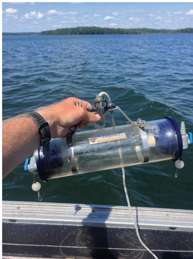
A Van Dorne Sampler used to collect water samples from the bottom of the lake.
